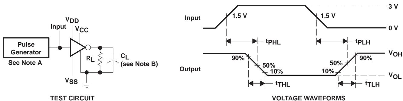
NOTES: A. The pulse generator has the following characteristics:  $t_w = 25\ \mu\text{s}$ ,  $\text{PRR} = 20\ \text{kHz}$ ,  $Z_O = 50\ \Omega$ ,  $t_r = t_f < 50\ \text{ns}$ .
